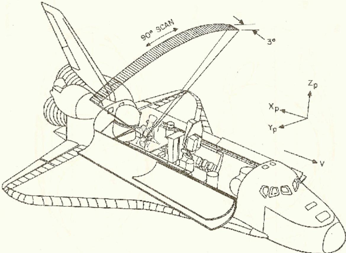
**Spacelab 2 Infrared Telescope**
