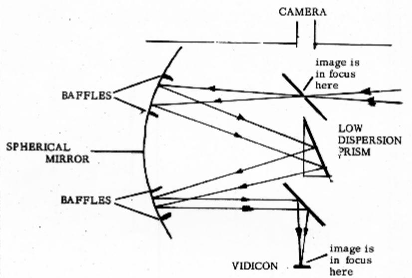
MIT Vidicon Spectrometer with camera monitoring slit in mirror
