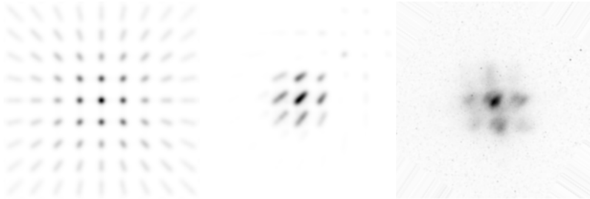
Fig. 3.6.— Numerical simulation of PSF for the instrument (left ) with the pupil densifier removed (Fizeau mode), in densified-pupil mode on a dispersed order (centre) and the star \alpha Gem (right). Comparing the star image to the numerically simulated PSF we deduced that pointing errors positioned the object outside the field of view of the interferometer. The result is a dispersed image of the double star.
