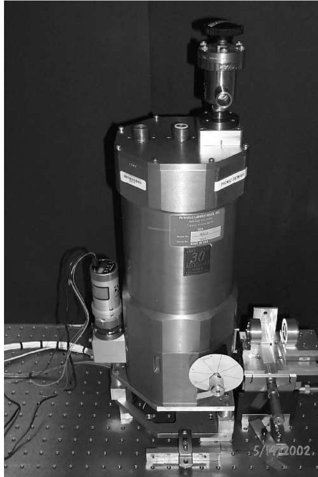
Fig. 4.3.— The PICNIC camera dewar and the optics focusing the beams from the IONIC3T beam combiner are shown in this picture. The mechanical assembly is an improved version of the previous NICMOS3 design, but the dewar is taller and contains more liquid nitrogen, one extra filter wheel is implemented, (in order to insert density filters), and both filter wheels are able to be motorised.
